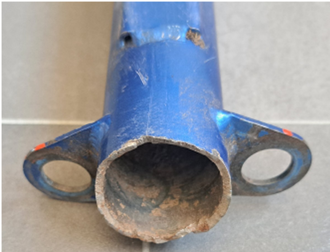
Figure 2 The fracture surface at the end of the leg.
