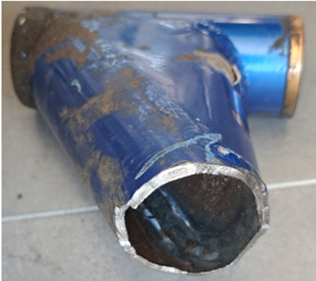
Figure 3 Fracture area on the lower broken part of the leg
