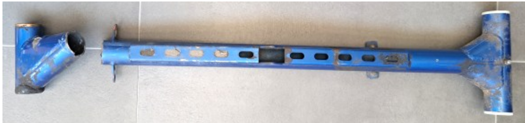
Figure 1 Front undercarriage leg with broken lower end.
