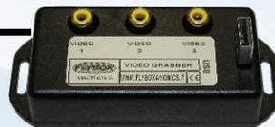
Up to 3 color cameras can be connected to Vigilus through the Video Grabber, to monitor your landing gear or under belly insights of the aircraft.
